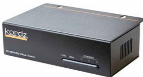
Above: Kordz's PLX-HDB.4 HDBaseT Extender enables the transport of uncompressed high speed HDMI, six-port Ethernet, IR, and RS232 data simultaneously over a single Cat-5e/6 cable up to 100m.
